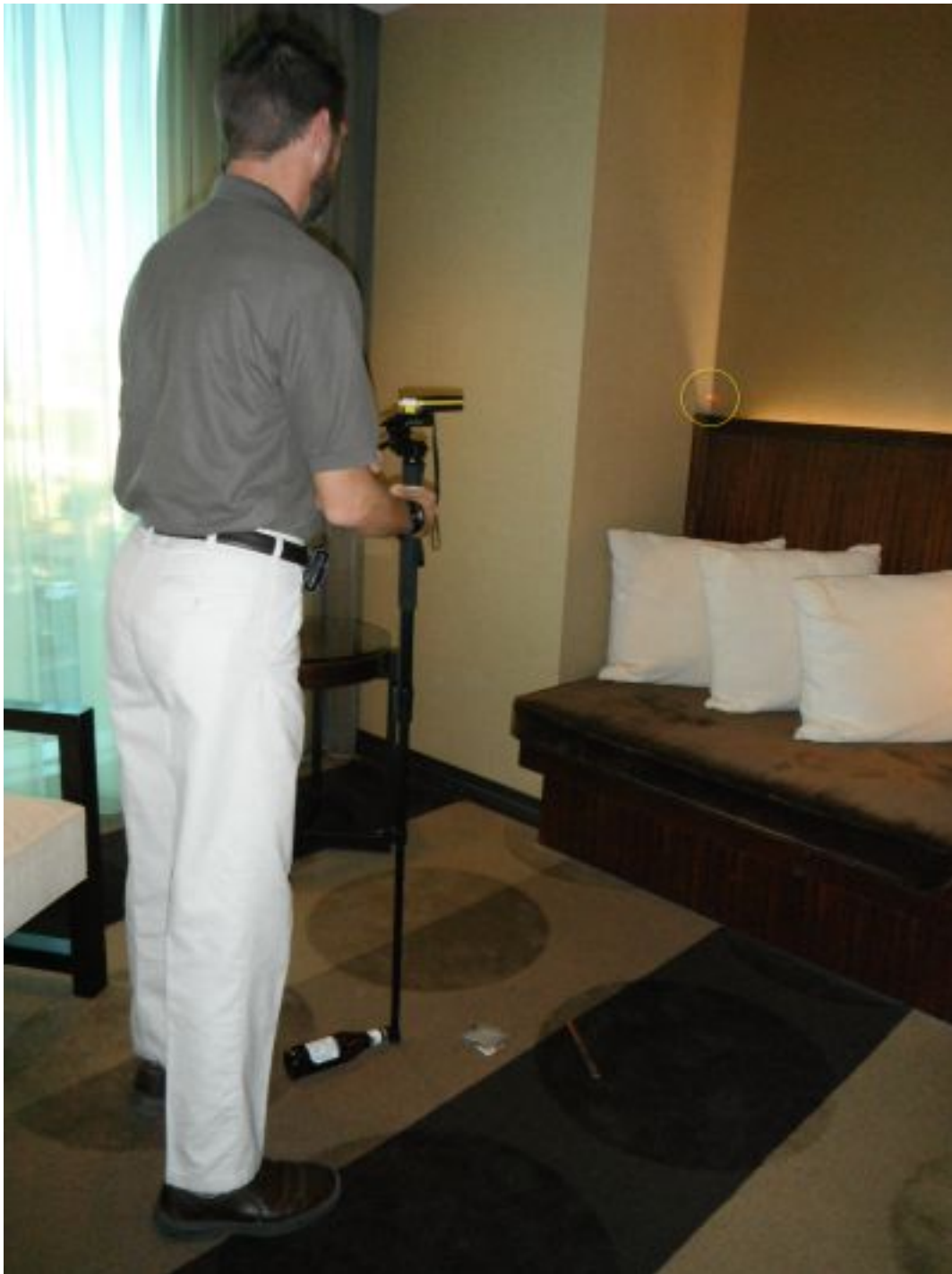
Photo 3: Using a laser measuring device and a monopod to measure from the beer bottle to the control point (corner).
